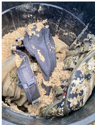
↑ All packs passed the sand-in-the-zippers test without sticking or breaking.
